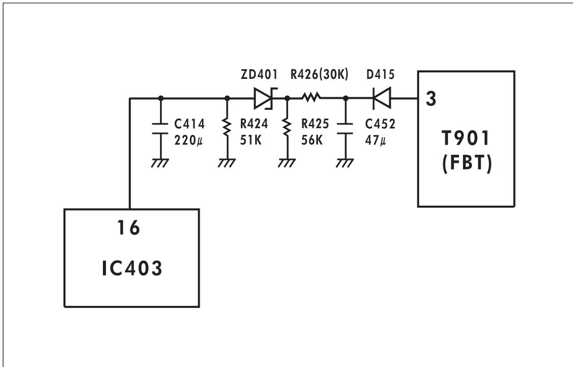
The pin 3 of the flyback transformer supplies feedback voltage to the X-ray protection circuit..
